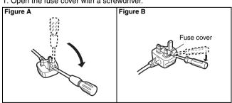
2. Replace the fuse and close or attach the fuse cover.
